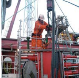
A wireline operator preparing a tool for deployment on StatoilHydro's Heidrun platform, Haltenbanken.
