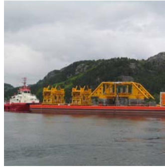
Sail-away of Morvin manifold and Lavrans templates, manufactured at Aker Solutions' facility at Egersund, Norway.
